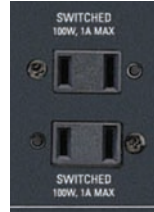
Figure 21 – Switched AC Accessory Outlets
